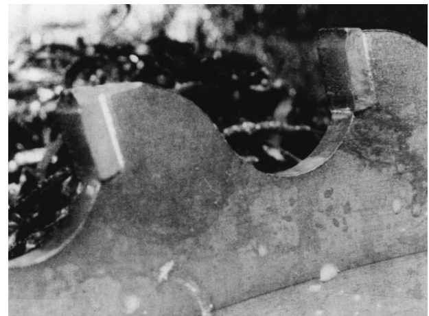
Fig. 12. Ti–C–N-coated tips after cutting 3.4 m 2 of hard steel, showing good adhesion and wear resistance of the coating.
